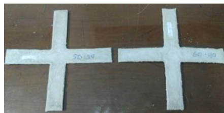
Gambar 2. Rangka drone berbahan green composite material
