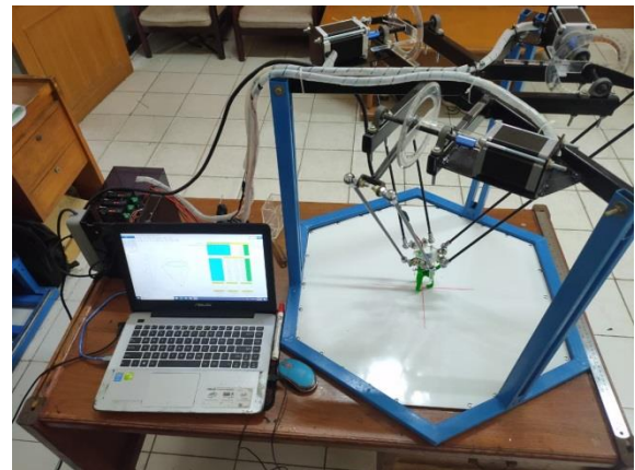
Gambar 1. Rancangan Manipulator Paralel 3-RRPaR
