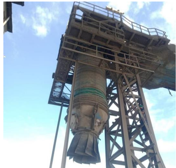
Gambar 12. Cone Chut Telescopic Shiploader
