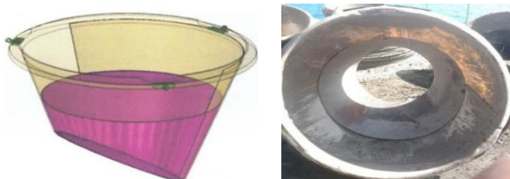
Gambar 11. Cone dilapis Plat Baja 3 mm
